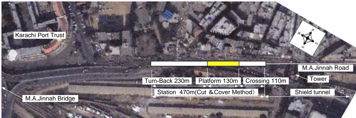
Figure A1-3-33 Terminal Station Plan (Tower Station)
